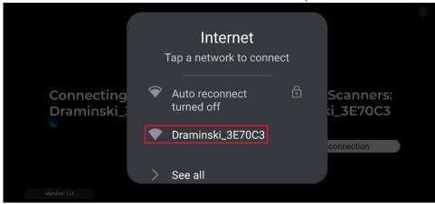
If you don't see the network created by your ultrasound scanner, make sure the Access Point (WiFi AP) is enabled in the ultrasound settings. If that doesn't help, disconnect and reconnect the WiFi antenna.
