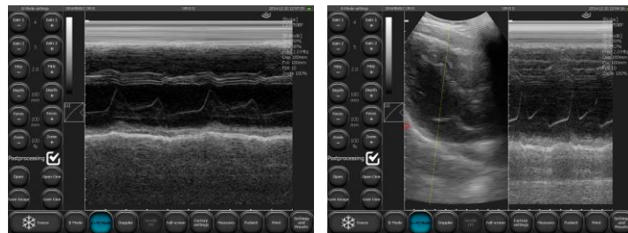
Fig. 17 Imaging modes: M and B+M
