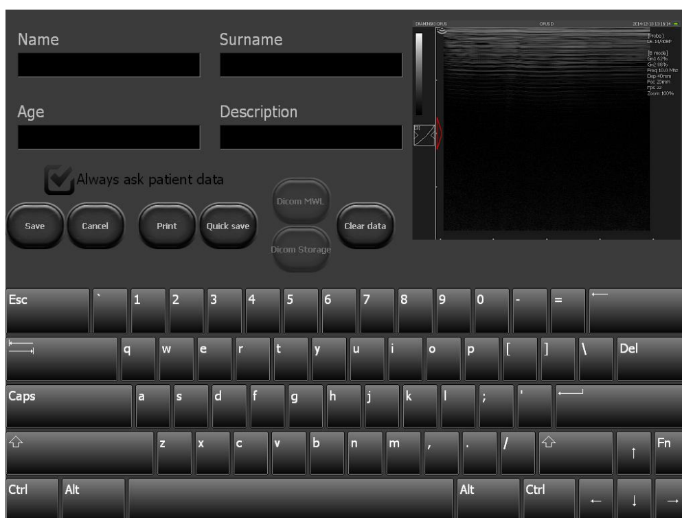
Fig. 25 Dialogue box used to enter patient's data during image / cine loop saving
