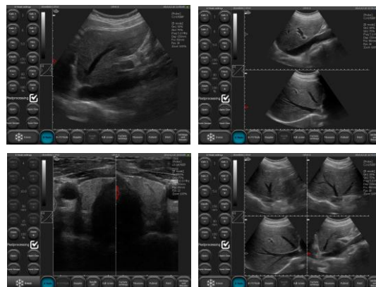
Fig. 16 Imaging modes: B, B+B and 4B
