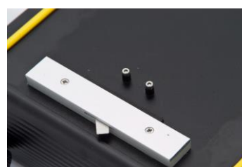
Photo 3. Strap and terminals for battery
